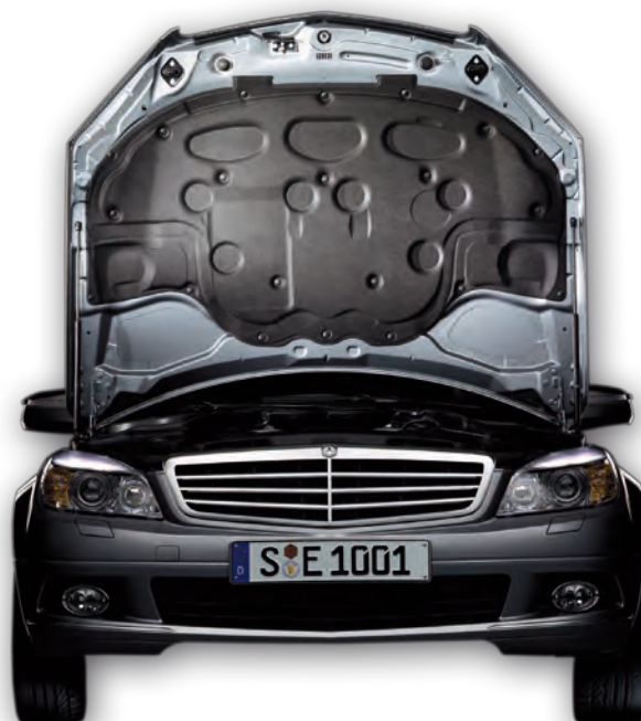
Basotect component of Carcoustics, D in the Mercedes C class. Photo: Daimler AG, D
