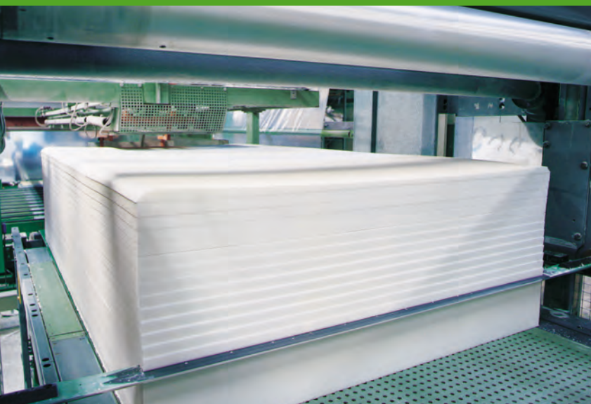
Cutting of Basotect® panels
